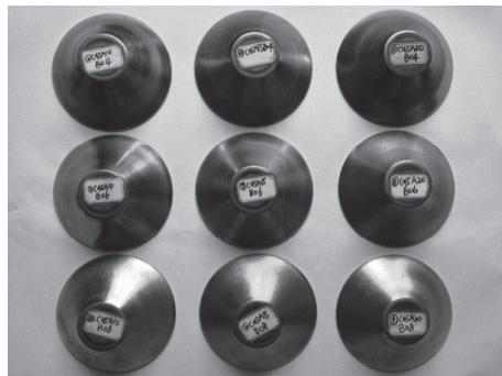
图14 GH3030 高温合金薄壁锥形钣金旋压件 Fig. 14 Thin wall conical spinning parts of GH3030 superalloy
